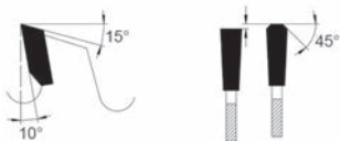
Flach-Trapezzahn Flat trapezoidal tooth
