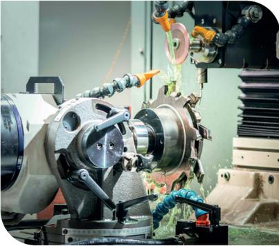
Compared to HSS tools or carbide-tipped tools, PCD-tipped tools do not wear by rounding; instead, the cutting edges or segments break out as usage progresses.
