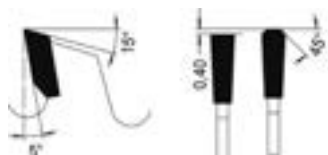
Trapez-Flachzahn Trapezoidal flat tooth
