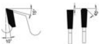
Trapez-Flachzahn Trapezoidal flat tooth
