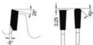
Trapez-Flachzahn, negativ Trapezoidal flat tooth, negative
