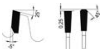
Trapez-Flachzahn, negativ Trapezoidal flat tooth, negative
