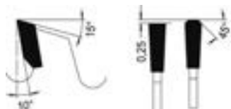
Trapez-Flachzahn Trapezoidal flat tooth
