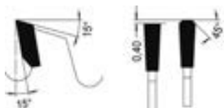
Trapez-Flachzahn Trapezoidal flat tooth
