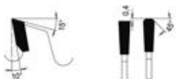
Trapez-Flachzahn Trapezoidal flat tooth
