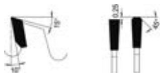
Trapez-Flachzahn Trapezoidal flat tooth
