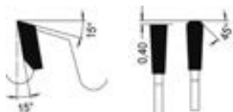
Trapez-Flachzahn Trapezoidal flat tooth
