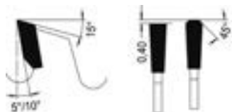
Trapez-Flachzahn Trapezoidal Flat tooth
