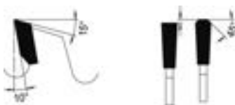
Trapez-Flachzahn Trapezoidal flat tooth
