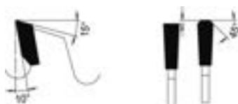
Trapez-Flachzahn Trapezoidal flat tooth
