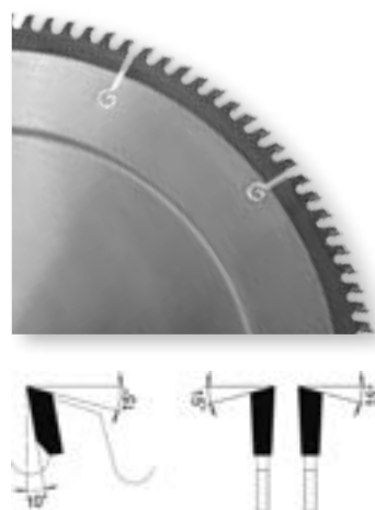
Wechselzahn Alternate top bevel tooth
