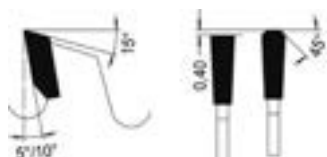
Trapez-Flachzahn Trapezoidal Flat tooth
