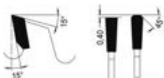
Trapez-Flachzahn Trapezoidal flat tooth
