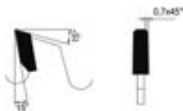
Trapezzahn Triple chip tooth
