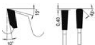
Trapez-Flachzahn Trapezoidal flat tooth
