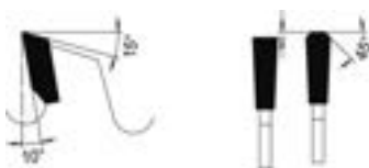
Trapez-Flachzahn Trapezoidal flat tooth
