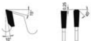
Trapez-Flachzahn Trapezoidal flat tooth
