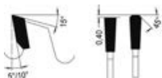
Trapez-Flachzahn Trapezoidal Flat tooth
