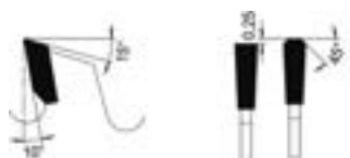
Trapez-Flachzahn Trapezoidal flat tooth
