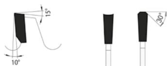
Hohlzahn-Dach-Flach Hollow inverted V/flat tooth
